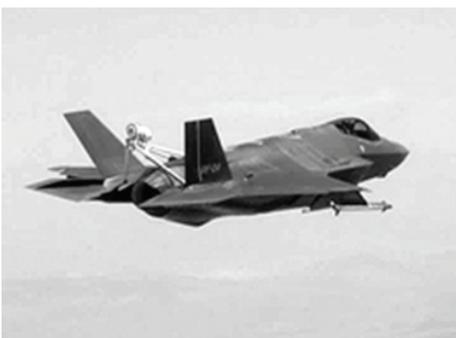
weapon bay doors. The F-35A began edge-of-the-envelope high AOA testing in the Fall 2012. For all testing, recovery from out of control flight has been 100 percent suc-
