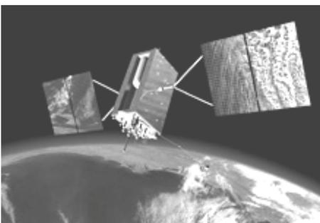
The recent testing of GPS III space vehicle 1 (SV 1) bus – the portion of the space vehicle that carries mission payloads and hosts them in orbit – assured that all bus subsystems are functioning normally and ready for final integration with the satellite’s navigation payload. Systems tested included: guidance, navigation and control; command & data handling; on-board computer and flight software; environmental
