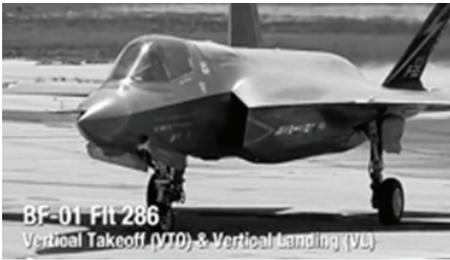
capabilities required for the fielding an F-35B aircraft. While not a combat capability, VTOs are required for repositioning of the STOVL in environments where a jet could not perform a short takeoff. In these cases, the jet, with a limited amount of fuel, would execute a VTO to travel a short distance.
