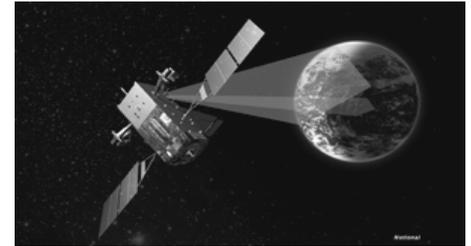
SBIRS GEO-1 includes highly sophisticated scanning and staring sensors that deliver improved infrared sensitivity and a reduction in area revisit times over the current constellation. The scanning sensor provides a wide area surveillance of missile launches and natural phenomena across the earth, while the staring sensor can be tasked to observe smaller areas of interest with superior sensitivity. GEO-1 transmitted its first infrared image on June 21.
