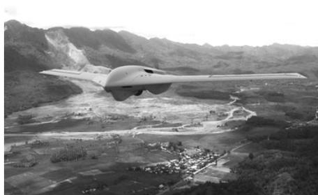
*Lockheed Martin's Fury unmanned aerial system (UAS) has reliably demonstrated more than 12-hour endurance, while simultaneously operating 100 pounds of ISR (Intelligence, surveillance, and recon) payloads.*
