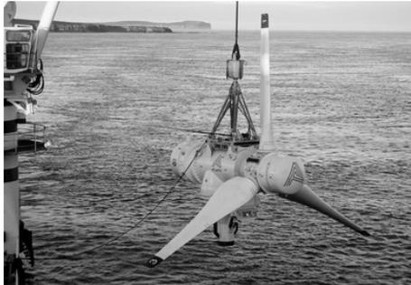
Lockheed Martin developed, manufactured and delivered two innovative subsystems, the Yaw Drive System (YDS) and the Variable Pitch System (VPS). The two elements enable the turbine to rotate autonomously around its base, so it always faces into the tidal flow. The pitch angle of the turbine blades also adjusts to optimize the power generation in a given tidal stream.
