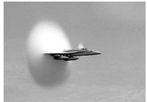
**Aerodynamic condensation evidences of supersonic expansion fans around a transonic F/A-18**
