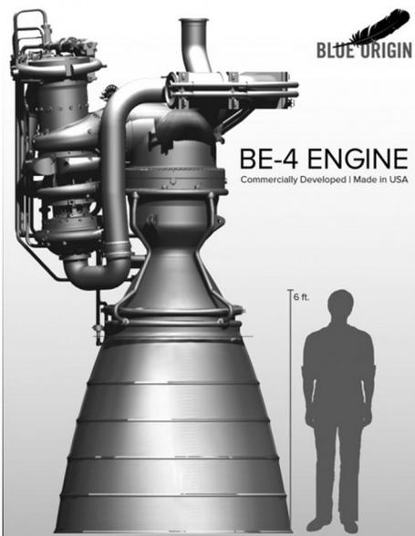
In addition to replacing the RD-180, the BE-4 is designed to power Vulcan, ULA's next generation launch vehicle. Two BE-4s would power each ULA Vulcan booster, providing some 1,100,000-lbf (4.9 MN) of thrust at liftoff. Vulcan will launch from Space
