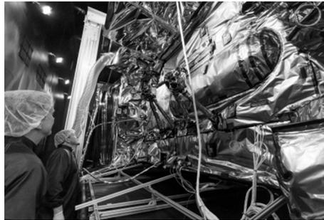
*The first GPS III satellite recently completed system-level Thermal Vacuum testing, validating Lockheed Martin's design for the next generation of more powerful GPS satellites.*
