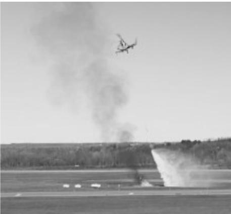
*The unmanned K-MAX drops water on a fire during a demonstration at Griffiss International Airport in Rome, New York. The Indago quadrotor identified hot spots and relayed that information to an operator who directed the K-MAX to autonomously retrieve water from a nearby pond and drop it onto the fire*
