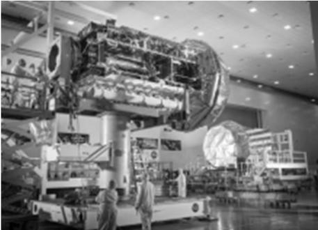
The MUOS satellite was stressed at extreme hot and cold temperatures in a vacuum at Lockheed Martin's Dual Entry Large Thermal Altitude chamber, simulating the environments the satellite will experience throughout its mission life.
