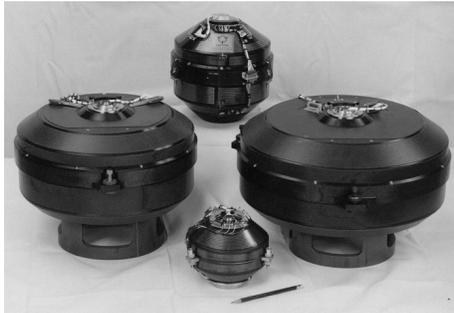
Lockheed Martin builds multiple versions of gravity gradiometer instruments, like those (top center) used in Full Tensor Gradiometer (FTG) systems. Other gradiometers (left and right) are used for partial-tensor systems, such as the CGG Falcon™ and the Land Gradiometer System, while smaller instruments (bottom center) are targeted for navigation applications.
