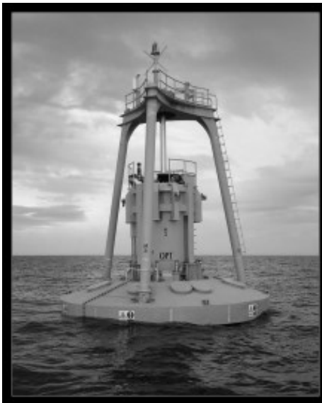
Wave power uses special buoys that use the rising and falling of ocean waves to generate electricity. Photo courtesy Ocean Power Technologies, Inc.
