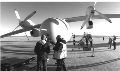
The unmanned plane has a wingspan of 150 feet and is capable of carrying a 450-pound load. Even though 5 hours is one of the longest flights ever for the prototype (early model) aircraft,
